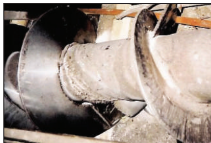
Abraded screw conveyor.
