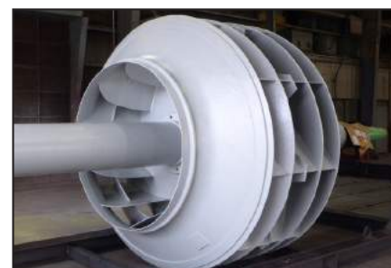
Dynamically balanced ARC S7 AR coated fan.
