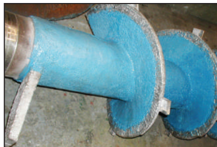
ARC MX1 applied and tips welded.
